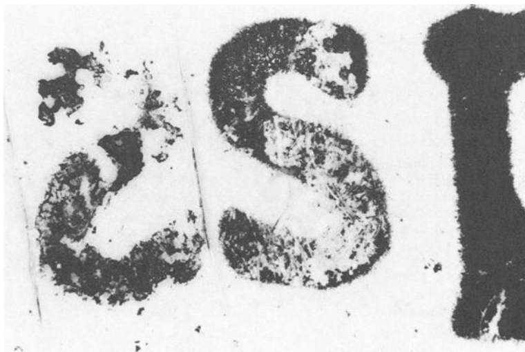
FIG. 1—A sample lifter (the glass rectangle with the backwards letter "s") has been used to remove a portion of the toner from the letter "s" displayed. A fiber is visible which has been ripped up from the page in the process (shown at about \times 40 magnification).
